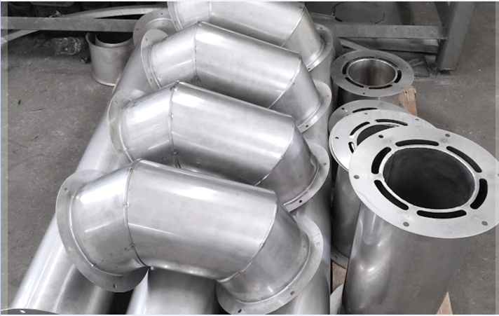
WELDED STAINLESS DUCT AND FITTINGS
