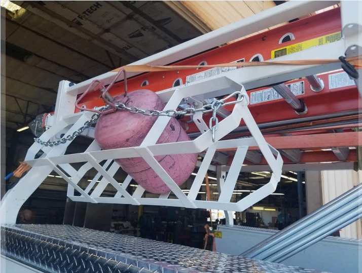
REFRIGERANT TANK STORAGE RACKS
