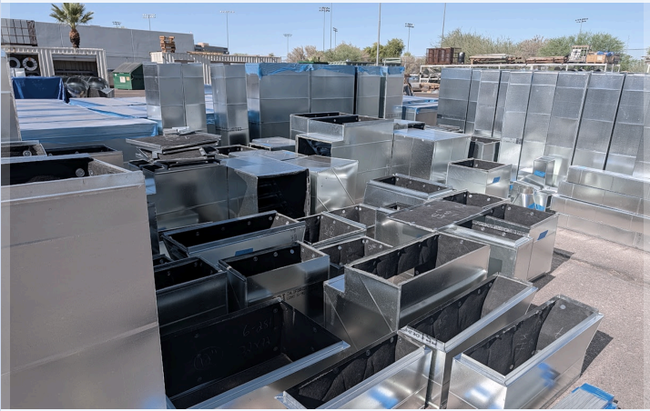
MECHANICAL LOCK SEAM DUCTWORK
