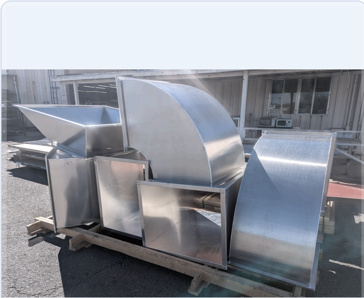
ALUMINUM MECHANICAL DUCTWORK
